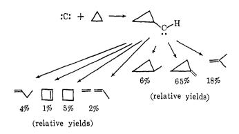
There were also isomeric C<sub>6</sub> materials, presumably radical coupling products, but no acetylene was formed. This is unlike the reactions of 2-methylpropane and cyclopropane with carbon atoms produced by nuclear processes where acetylene is formed to the extent of 21.2 and 42.7%, respectively, in oxygen-scavenged systems.<sup>5</sup>
